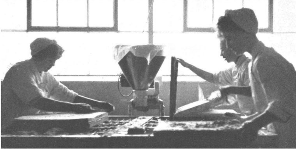
The girls at work on the left are preparing large sheets of sponge cake which will be used to make J.S. Coconut Iced Cake. The cakes must have the fine layer of brown crust removed from them before they are stacked and cut into long square sectioned strips.
