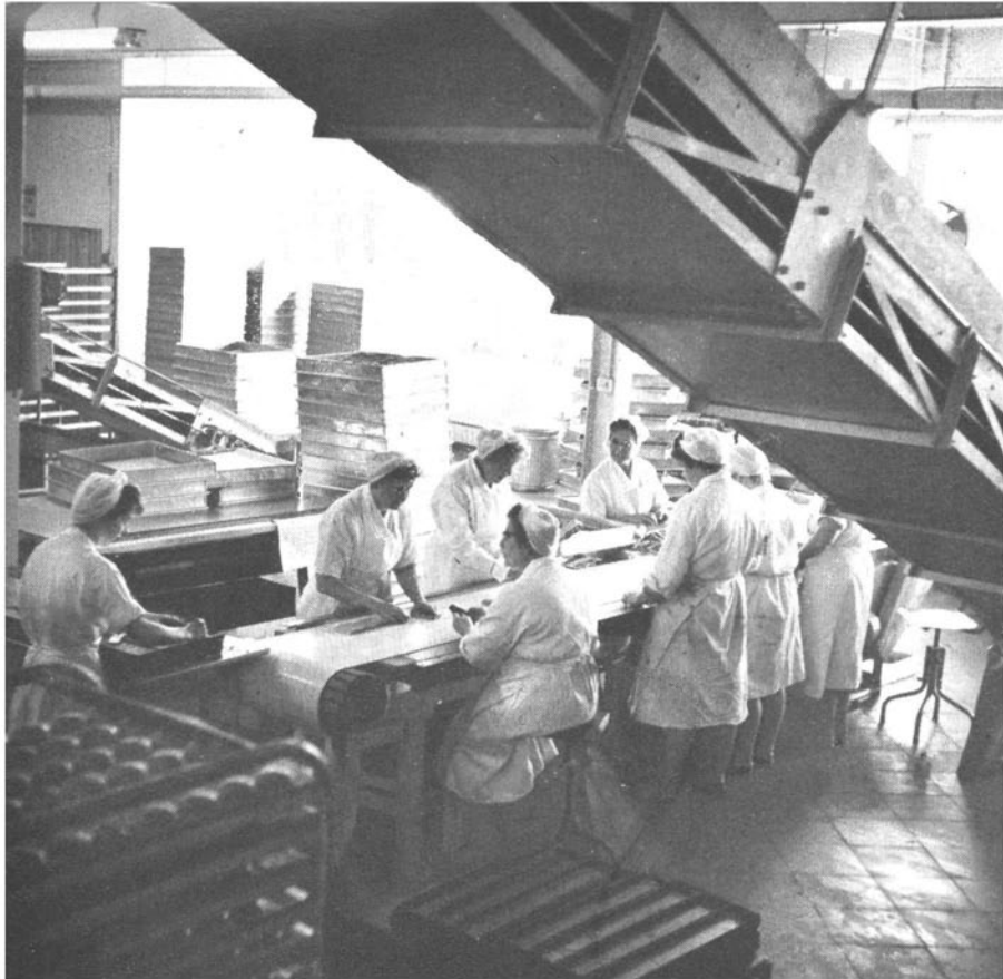
At the far end of the ovens are packing tables for some lines, but others go up to the first floor on boxed-in conveyor belts. As they come up one of the staff stacks them on shelves ready for the next processing. It may be chocolate coating done by an "enrobing machine" or turning into a "sandwich" and decorating with confectionery ornaments.
