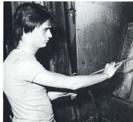
In the printroom Tim Wood uses a powerful water jet to clean the screens.
