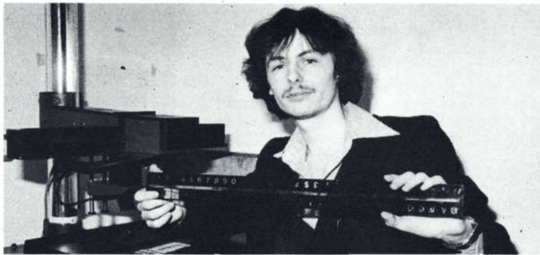
Master negatives like the one Colin Purnell is holding cost about £60 each. It is from these masters the 'copy' is made up on the photo-composing machine behind.
