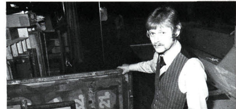
Screens can be stored for repeat runs. Here Stan Norton shows us what a blank Polyester screen looks like against one with a stencil in position.
