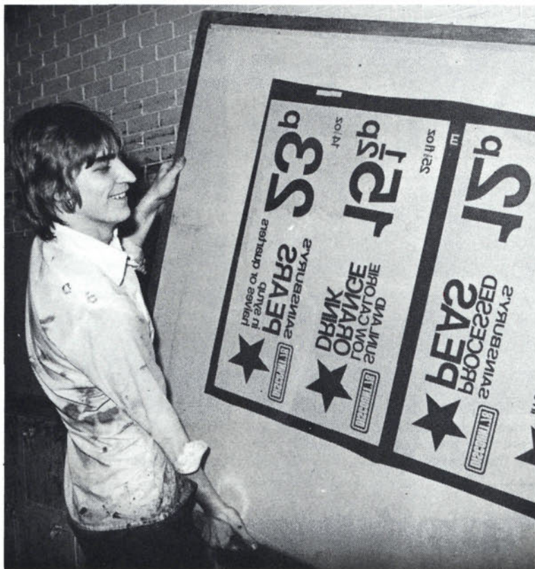
Mick Lynch puts a screen to dry. The next step will be to 'spot out' any imperfections and peel off the stencil backing film.
