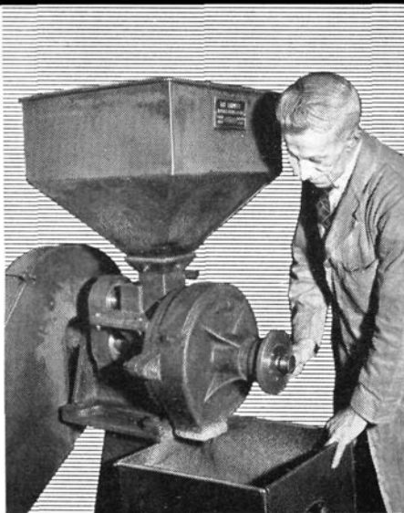
Once cool they are ground. The grinder gives fine or coarse results as required.
